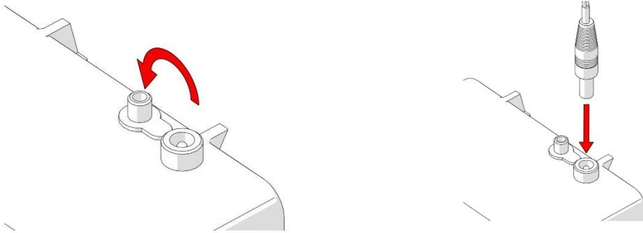
9. Connect transformer (mains powered) as shown, check for leaks and test tap for correct operation. If using battery powered option, refer to “FITTING OR REPLACING BATTERIES”.
